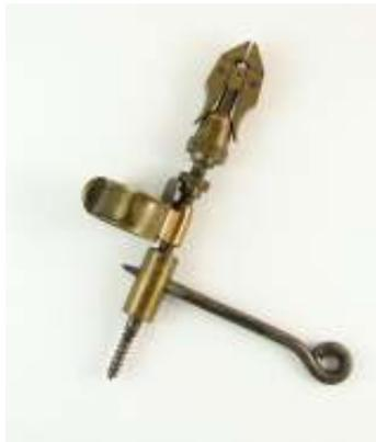
This Vise is pictured in The 1909 Hardy Brothers Catalog and can be worn on The thumb or screwed into a suitable surface for use. It measures just 4” from end to end.
