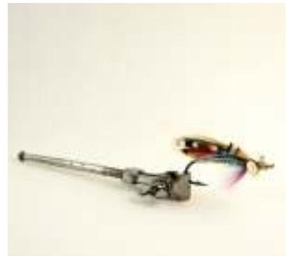
A 4.25” Victorian Era Hand Vise. Note The Two-Piece, hinged jaws and the Nickle plating. The handle is solid, whereas they are almost always hollow.
